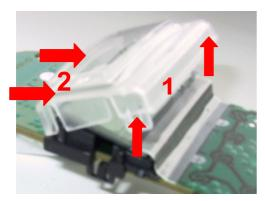
Snap the 2 hooks on the bottom open (1). Then lift the display carefully until the 2 snap hooks on the top open (2).
