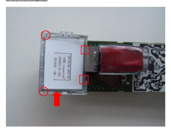
Insert the opening tool G2000 between both plastic parts (cover and bottom) and press down in order to open the first hook (red rectangle).
