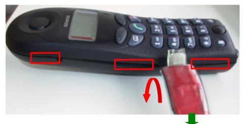
Insert opening tool G2000 in the above described position between both hooks (red rectangles). After inserting push the tip of the tool downwards (red arrow) and press the other end down (green arrow) in order to lift the upper case shell. If necessary insert a second opening tool G2000 in the hook area (red rectangles) and try so to lift the upper case shell.
