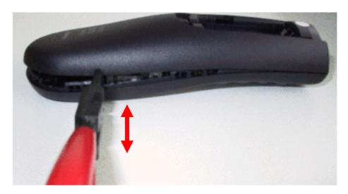
Insert pliers in belt-clip-hole and press to open upper part of the housing. Do the same in the other belt-clip-hole.
