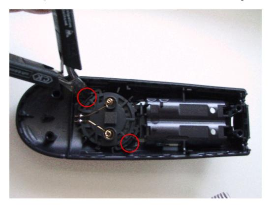
Just remove snap hooks (red circles) with a sidecutter and lift loudspeaker.
