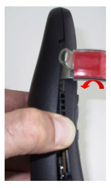
Insert the tool in the above described position and try to disengage the belt clip hook (red circle) by pressing it downwards. Do the same on the opposite side of the handset.
