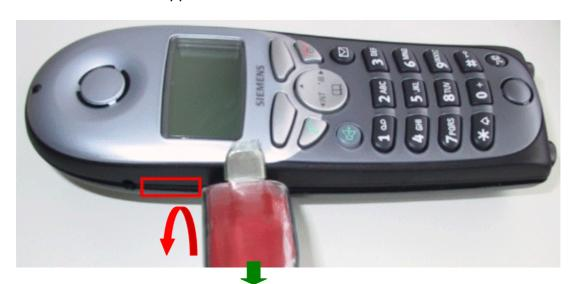
Insert the tool in the above described position and try to disengage the belt clip hook. Do the same on the opposite side of the handset.
