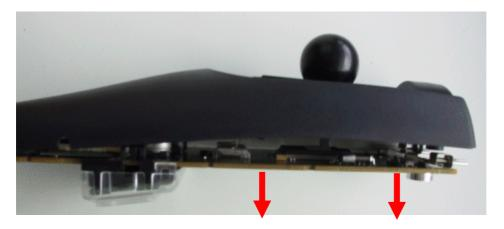
Insert battery dummy G3000 in battery compartment. Pull the board evenly in order to get upper and lower spring at the same time out of the battery compartment.
