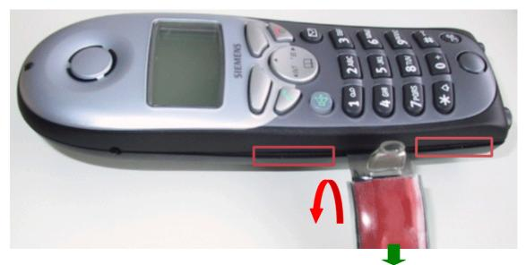
Insert opening tool G2000 in the above described position between both hooks (red rectangles). After inserting push the tip of the tool downwards (red arrow) and press the other end down (green arrow) in order to lift the upper case shell. If necessary insert a second opening tool G2000 in the hook area (red rectangles) and try so to lift the upper case shell.
