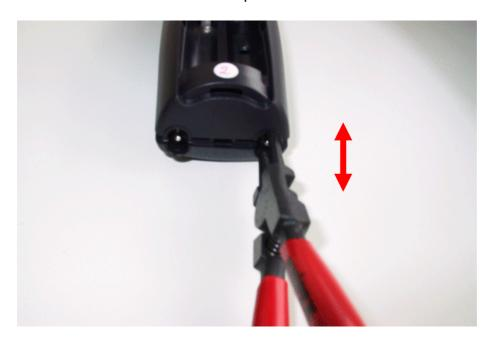
Insert pliers in charging-contact-hole and press to open lower part of the housing. If necessary do the same in the other charging-contact-hole.
